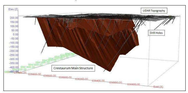
Figure 14-5 Isometric View Looking Northwest: Distribution of the Drill holes, Sam Otto,
