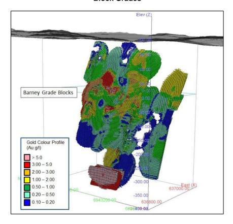
Figure 14-11 Isometric View Looking Northwest of the Mispickel Deposit Mineral Resource Block Grades and Revenue Factor 1.0 Pits
