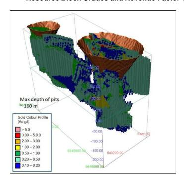
Figure 14-12 Isometric View Looking Down, Northwest and Northeast of the Sam Otto/Dave's Pond Deposit Mineral Resource Block Grades and Revenue Factor 1.0 Pits
