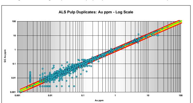
Figure 11-1 Log X-Y plot of ALS pulp duplicates of Gold Terra drill samples.
