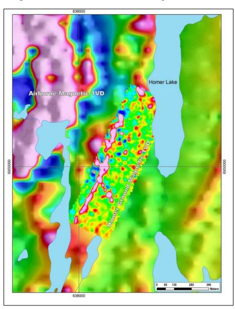
Figure 9-10 2015 Homer Lake Ground Magnetics Test – 1VD
