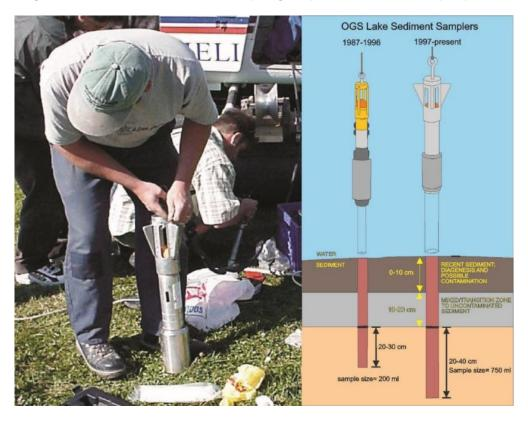
Figure 9-14 Lake sediment sampling torpedo unit and sample profile
