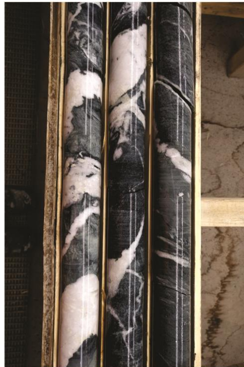
Figure 5 - Comparison of deformed quartz veining within the Campbell Shear (Figure 5A) in underground workings (5797 stope), and quartz veining in TCG20-064 at 523m within the interpreted Campbell Shear (Figure 5B)
