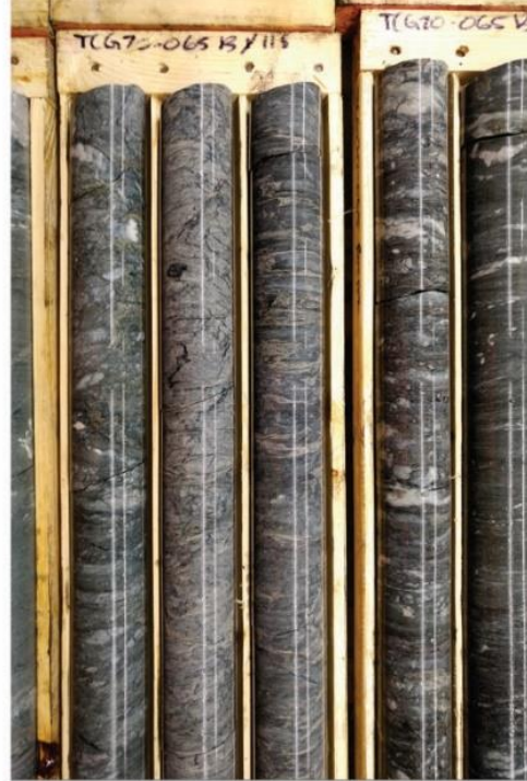
Figures 4-6: Comparison of alteration, quartz veining and sulphide mineralization from the Con mine (A) left side and Gold Terra drill holes within the Campbell Shear stratigraphy (B) right side.
